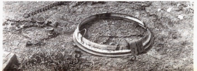
Gruntmier turns tires inside out by pulling this sawed-off tractor rim up through anchored-down tires (above) with a 3 pt. gin pole (shown below) mounted on his combine.
