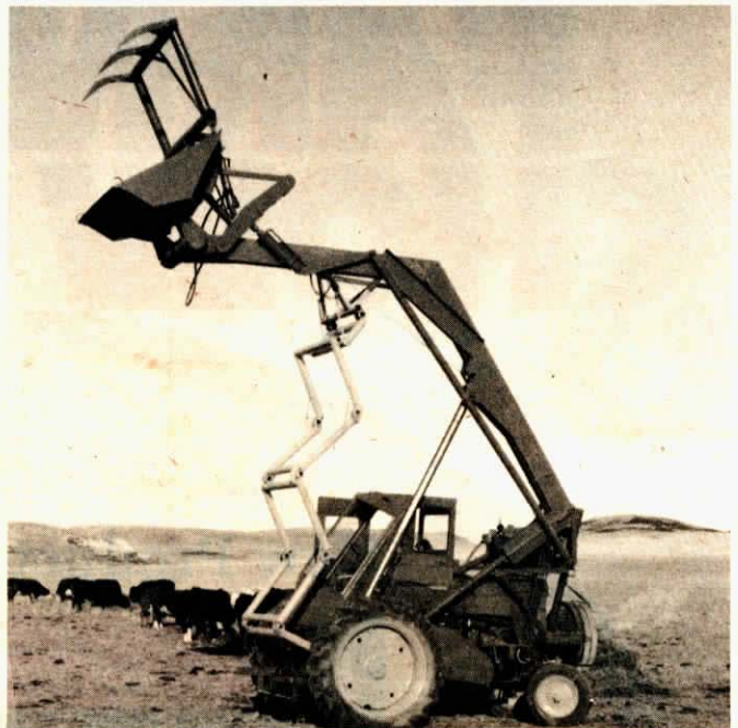
Support arms keep the small tractor from bouncing and jerking when the loader is fully extended.
