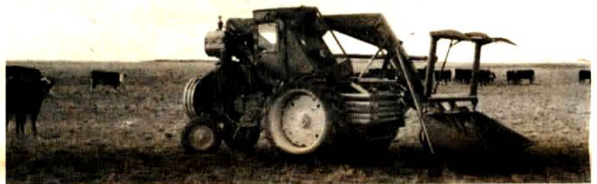
Hydrostatic tractor's unique loader support arms fold up neatly when bucket is lowered to the ground.
