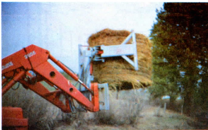
Bale forks mount on a 4 by 4 mast mounted above the loader mounting brackets.
