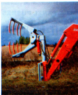
Cylinder mounted on mast turns bale grab forks 1/4 turn.
