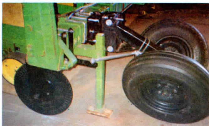
Tie rod runs from hinged V-wheels to pivoting coultter, which "steers" end of toolbar.
