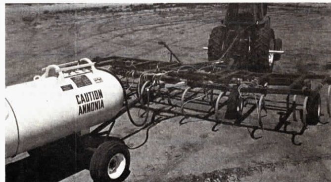
Ace Services will custom fit new anhydrous ammonia applicator kit to most any chisel plow, field cultivator or other tillage tool.
