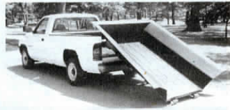
Rolling dump box installs in pickups.
