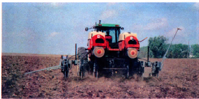
DeHaan decided to build his cultivator-planter when he was unable to buy one of Hiniker's new tag-along air seeders that rides on its own wheels behind the cultivator.
