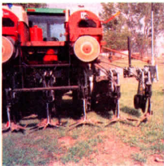
Air seed tubes run down the back of Hiniker's single sweep shanks and seed is deposited under the wings.
