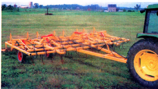
Steiner's cultivator has five rows of S-tines equipped with 2 1/2-in. sweeps.
