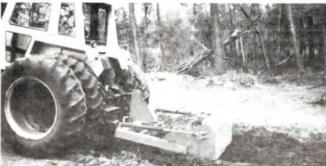
The 3-pt. scraper holds up to a yard of dirt and works great for such jobs as leveling driveways, scraping manure, and finish grading around buildings.
