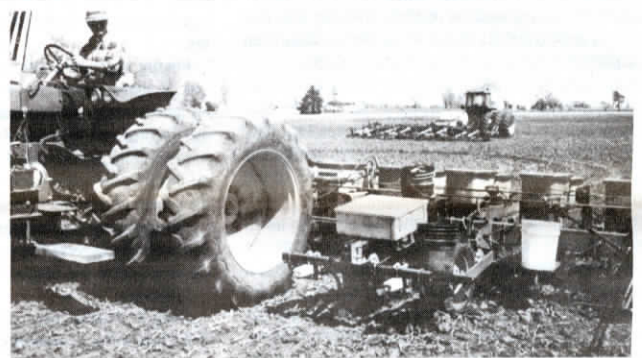
Cultivator shanks attach to short toolbar mounted ahead of planter. View from behind planter (below) shows side-by-side furrows that guide cultivator.
