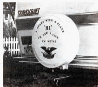
Metal disc, same diameter as tire, is placed over tire to lock it to vehicle.
