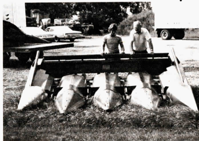
Wayne Weber narrowed-up this IH cornhead from 36 to 30-in. spacing.
