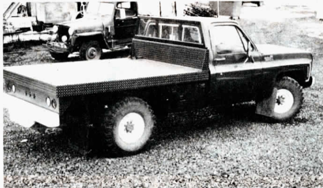
Truck bed fuel tank "V's" down between the rear truck frame to hold 260 gal. of fuel.
