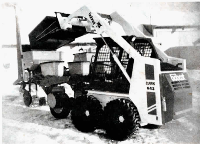
Hydraulic-operated door dumps Fast-Fill's load into planter boxes.
