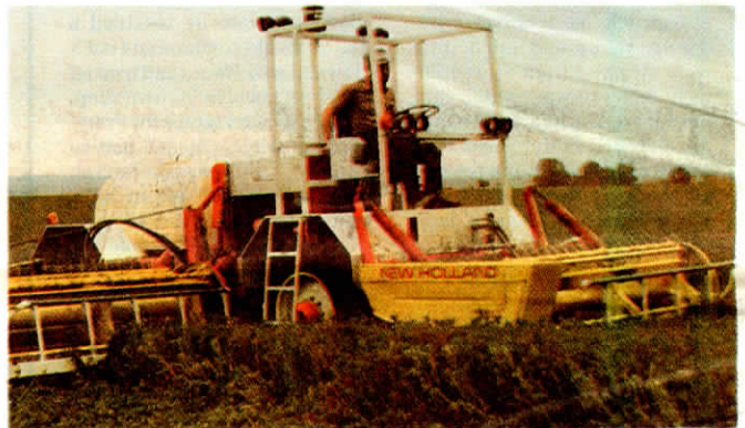
Spray attachments mounted on the front of each Haybine unit apply Pro-Cure, which dissolves wax on plant stems to speed drying.
