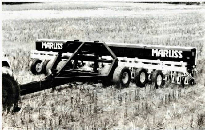
Caddy eliminates need for extra weight in cutting through heavy trash, residue.
