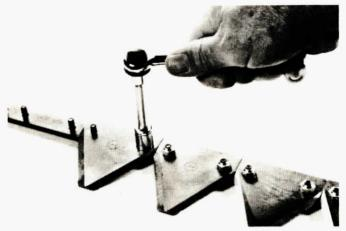
Bolts have splined ends so they don't turn as you tighten the nut.
