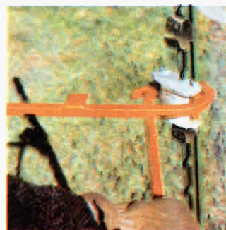
Magnetic tool head holds clip in the proper position. Diagonal opening for slipping wire out for quick take-down is adjustable for width.
