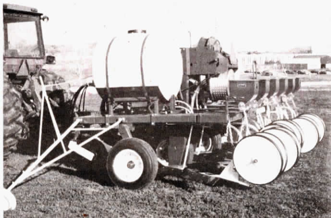
The Under Planter cuts out weeds, but leaves straw and stubble as an erosion-proof mulch.
