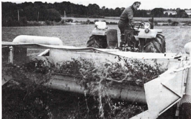
Air ducts at either end of new conditioner carry air under the pickup table where it gently lifts and conditions hay as it's cut.
