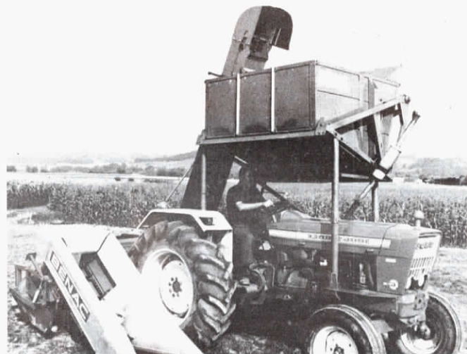
New for smaller European farms is this one row ear corn picker. Ears are elevated to a hopper mounted above the operator, eliminating the need to pull a wagon, or to hook and unhook wagons. Available with manually-operated down spout, or a hydraulically-operated dump. Contact: Albert Fontrier, General Manager, Berdoues, Mirande, 32300 France.
