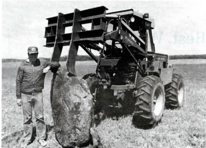
Frame of digger is made of 8 in. wide steel beam and the fork of 1½ in. thick steel plate.
