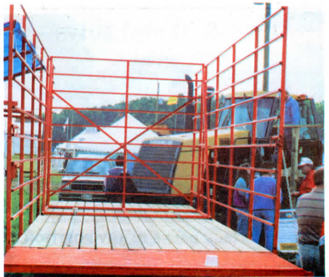
Back panel is skidded back and forth across deck of wagon by two steel cables controlled by electric-driven winch mounted under floor of wagon.
