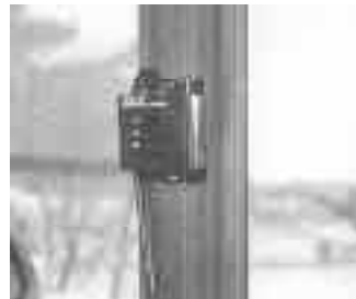
Add-on hydraulic system is engaged with a toggle switch in cab.
