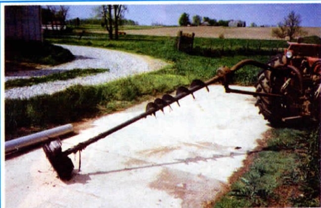
Car wheel "propeller" mounts at end of shaft attached to bottom of post hole auger.
