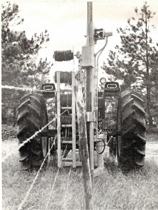
Fence Master strings up to five strands of barbed wire at a time, drives posts up to 10 ft. long and is self-leveling.
