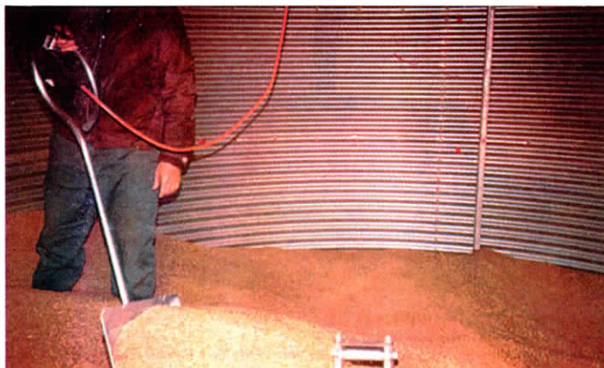
Special-built aluminum scoop shovel is tied to a poly cord threaded onto winch, which is mounted on unloading auger outside the bin.
