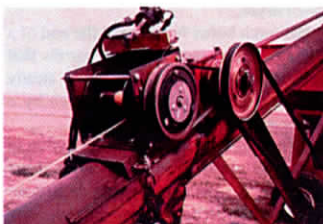
Winch is belt-driven off an add-on pulley on auger's gearbox driveshaft.
