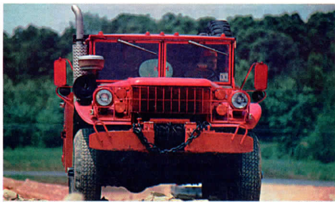
Truck is equipped with gear-driven winch "that has enough power to pull bellied-out dozers from swamps".
