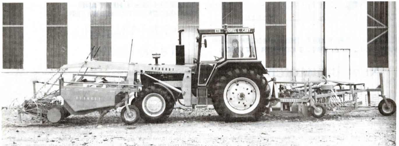
This version of Concord Front Linkage hookup on Deere tractor provides one-pass topping-windrowing and lifting of sugar beets. Note that extreme front "nose", used in hookup pictured above, has been removed for adapting Concord system for this particular hookup.
