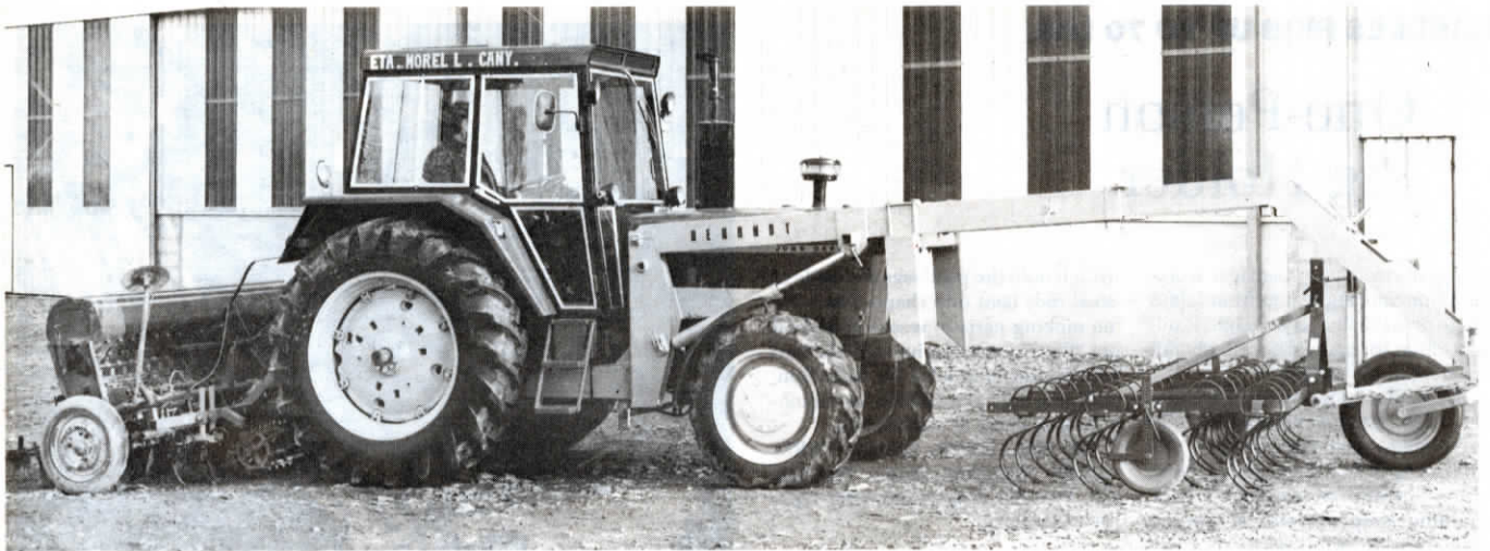
Standard 4 WD Deere tractor equipped with Dehandt Concord Front Linkage "nose job" attachment for simultaneous seedbed preparation and drilling. Long "nose" attachment allows front-mounted cultivator to be pulled rather than pushed.
