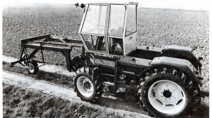
Converted 644 IH tractor from Dehandt is called the Autotractomatrice. Space behind the cab can be used for carrying a large chemical tank. Cab can be tipped up or removed for servicing.
