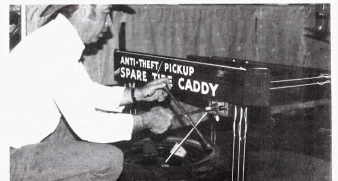
Tire wrench powers cable to pull tire in place under truck.
