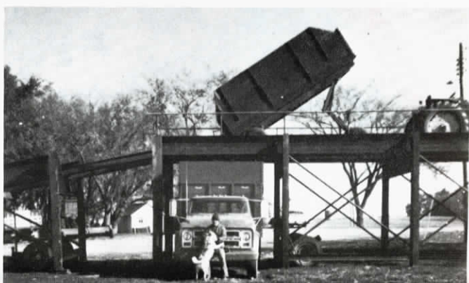
Note wheel to right of truck which is part of 3 pt. hookup for moving each section.
