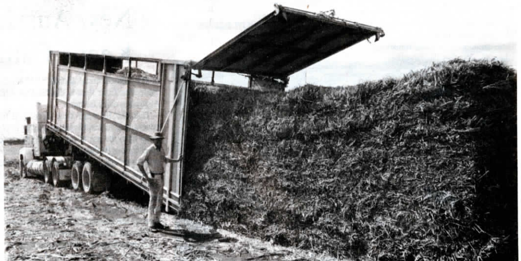
“It takes 2 to 3 hrs. to load an ordinary semi-load of square hay bales but you can load one of these 12-ton stacks onto a self-loading chain bed trailer in 5 min.,” says Terry McFarland.
