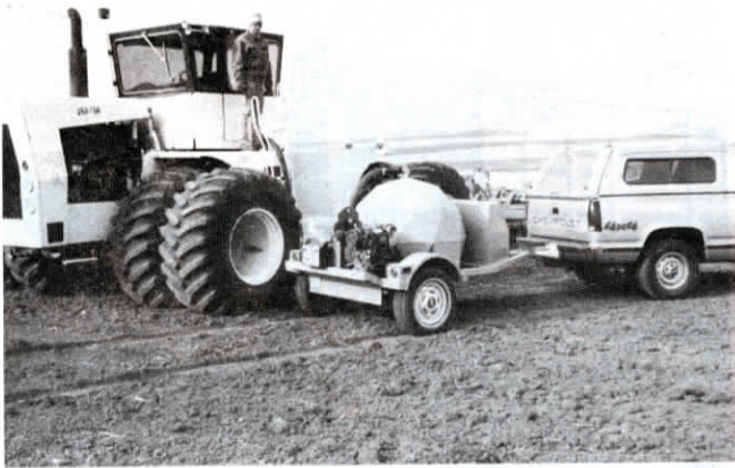
Geodesic 300-gal. fuel tank mounts on its own trailer, powered by a portable welder.
