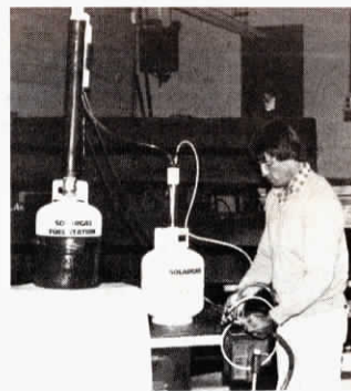
Spragg demonstrates the vacuum still kit with two small tanks. An ordinary garden hose and venturi valve create a vacuum inside the tanks, causing alcohol to boil at 120° instead of 170°.
