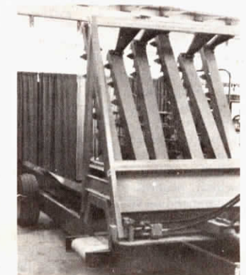
Six cutting arms cut each bale up, dropping hay to a belt and feeding it out the side.
