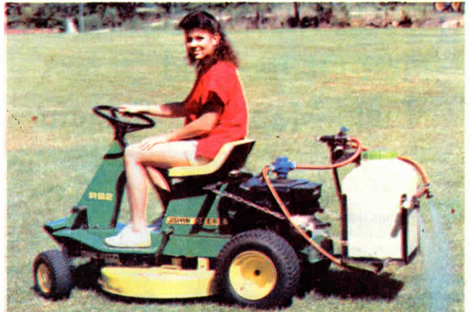
Coupler screws directly onto threaded end of crankshaft on lawn mower engines. The new 4-roller pump screws onto coupler and provides up to 200 psi spray pressure.
