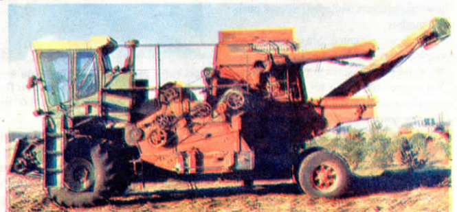
The two New Idea husking beds mount behind the cab and feederhouse. The sheller, which catches small ears that fall through the stalk-clearing rollers, mounts above and behind the husking beds.
