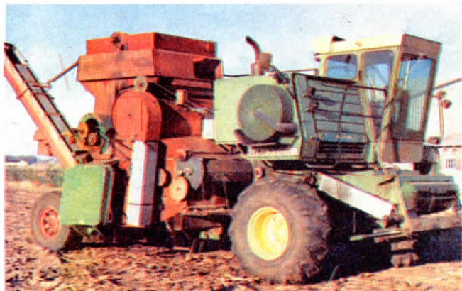
McGill removed the cylinder and concave on the Deere 7700 and everything behind them except for the bottom frame rails, which he extended 62 in.
