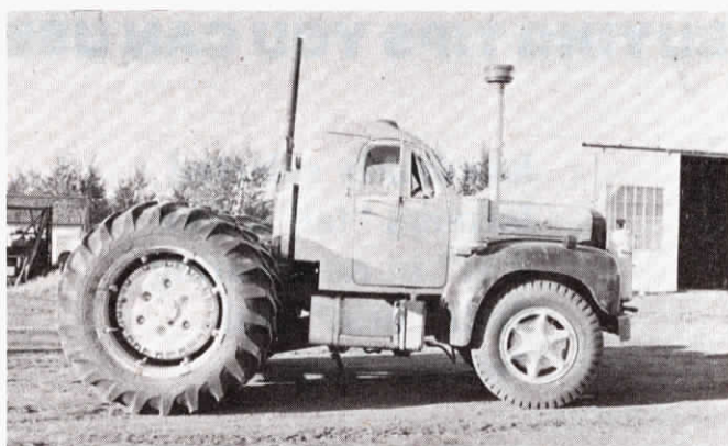
Tractor's cab, salvaged from the Mack truck, is cleaner and quieter than many conventional tractor cabs, say the Rasmussens.
