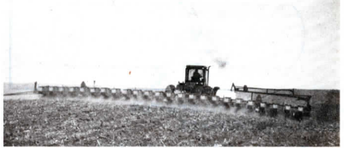
The planters are separated from each other so they can flex on sidehills.
