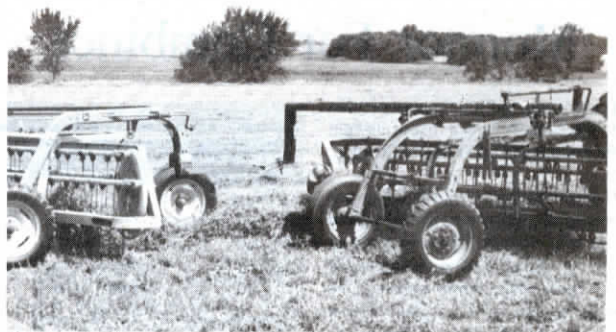
Center pole of a wagon gear is fastened to the frame of a New Idea 400 rake.
