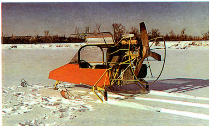
"Snow sled" rides on three 10-ft. long aluminum skis - two in back and one in front.
