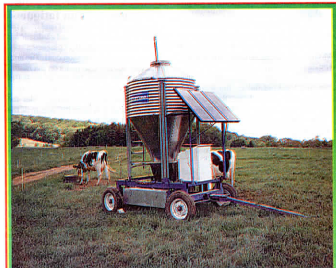
Rear-mounted, low-emissions 16 hp Briggs & Stratton "Vanguard" gas engine powers a 3-gear sectional pump that drives hydrostatic motors on each side.
