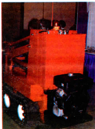
Rear-mounted, low-emissions 16 hp Briggs & Stratton "Vanguard" gas engine powers a 3-gear sectional pump that drives hydrostatic motors on each side.
