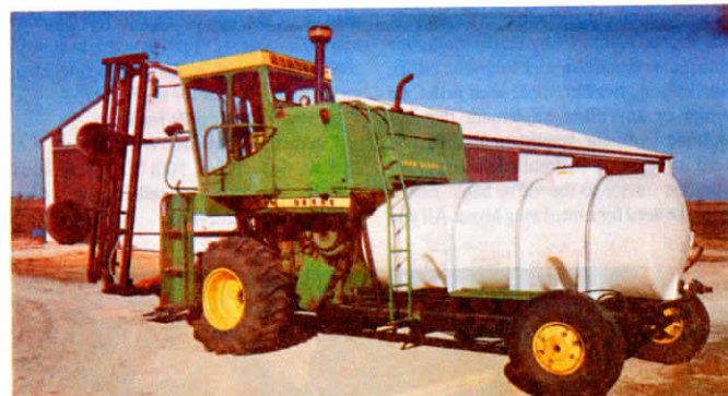
Spera built this self-propelled sprayer from a 1974 Deere 6600 combine.
