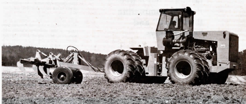
Rome Industries has introduced 375, 450 and 475 hp 4-wheel drive Rome tractors.
