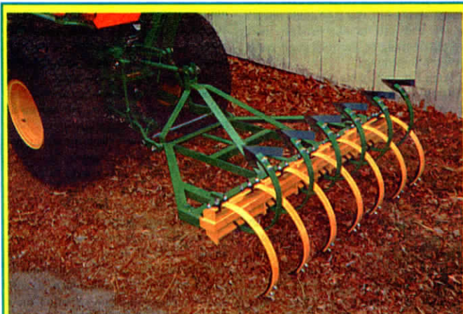
Freier's 2-way cultivator is fitted with a row of shanks fitted with sweeps and a row fitted with straight shanks.
