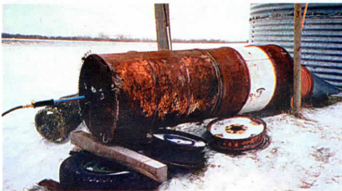
Propane torch burns full blast at end of a pair of welded-together steel barrels that bolt onto bin's aeration fan.
