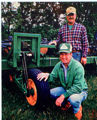
Photo courtesy The Farmer Magazine Ken and Howard Cotton moved transmission drive and gearboxes to the front of planter toolbar to reduce planter width.
