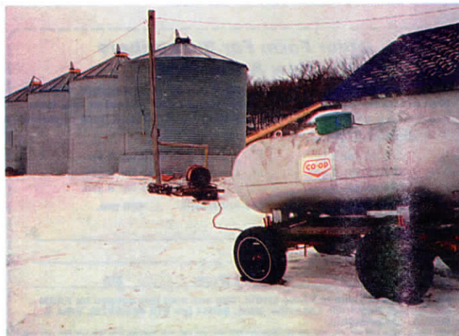
A steady flow of propane is fed to torch by trailer-mounted LP tank.
