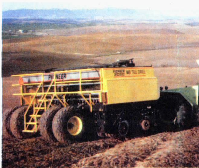
New Pioneer drill bands fertilizers and applies herbicides as it plants.
