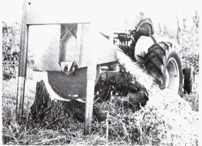
Stumpcutter handles stumps of any diameter up to 36 in. high.
