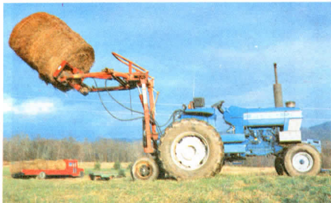
Crittenden put a bale spear on his squeeze-type Gehl bale mover and then mounted a set of dolly wheels underneath to carry weight of bale.
