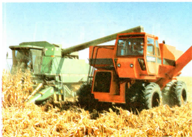
Blanchat designed the new grain cart from the ground up for speedy, efficient "spill-proof" hauling. Cart's 16-in. auger unloads 650-bu. hopper in less than 3 min.
