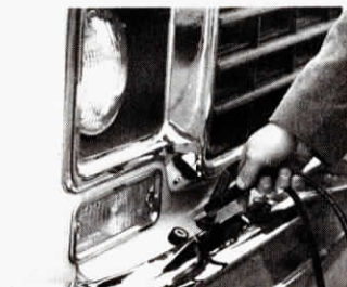
Close-up shows how male plug on Saf-T-Jump cable connects to terminals mounted on fender, behind bumper or wherever most convenient.
