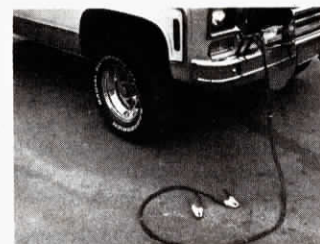
Cable with clamps on one end can be used to jumper vehicles not equipped with Saf-T-Jump battery-connect terminals on the fender or bumper.
