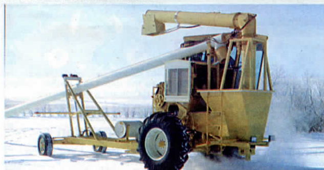
Rig is equipped with two augers - a long 40-ft. one that pulls grain out of storage and into a collection hopper, and a discharge auger that transfers grain to waiting trucks.
