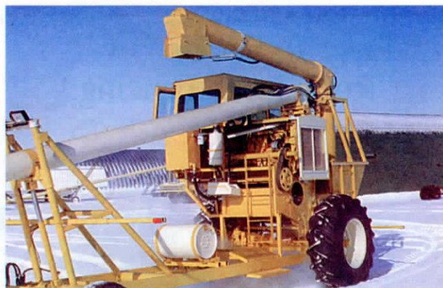
The auger is gas-powered by a late 1970's Massey Ferguson 410 combine engine.
