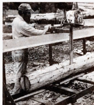
Chainsaw rolls down 16 ft. rack to cut logs into boards.
