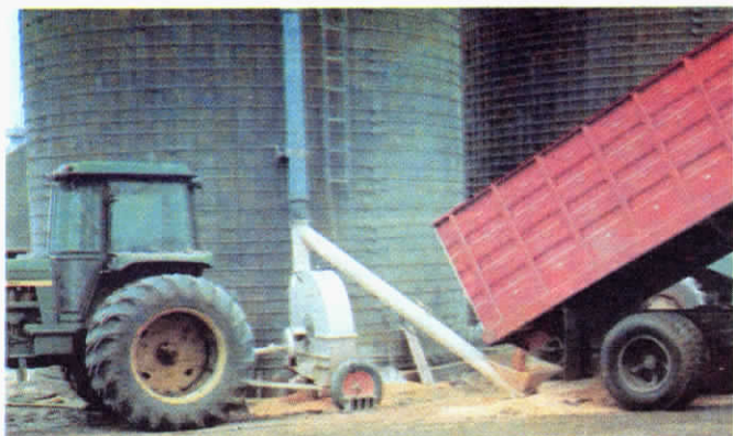
Bilyeu's silo blower blows dry or wet shelled corn, soybeans and other grains into silos 100 ft. and taller at the rate of up to 1,400 bu. per hour.
