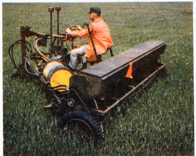
A 50 hp Volkswagen engine powers Lloyd Younger's self-propelled grain drill for planting soybeans in standing wheat.
