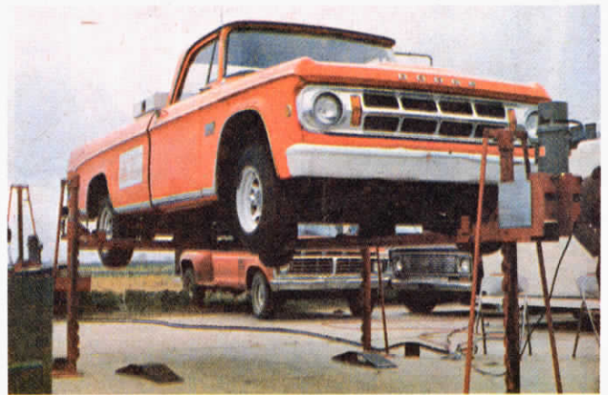
Portable hoist requires no air or hydraulic pressure. Uses an electric hoist that can lift up to 6,000 lbs.
