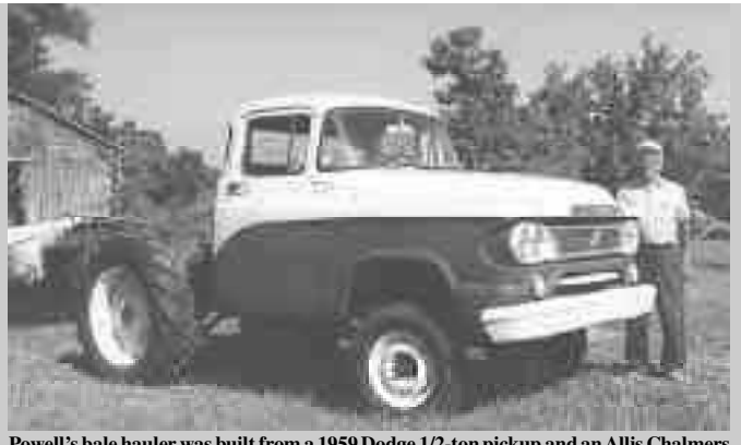
Powell's bale hauler was built from a 1959 Dodge 1/2-ton pickup and an Allis Chalmers WD-45 tractor.
