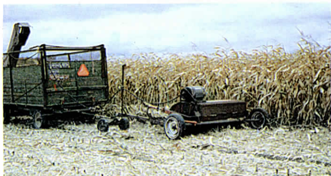
Schultheis pulls 6-ft. stalk shredder behind his New Idea 2-row corn picker and wagon. It shreds two rows at a time.
