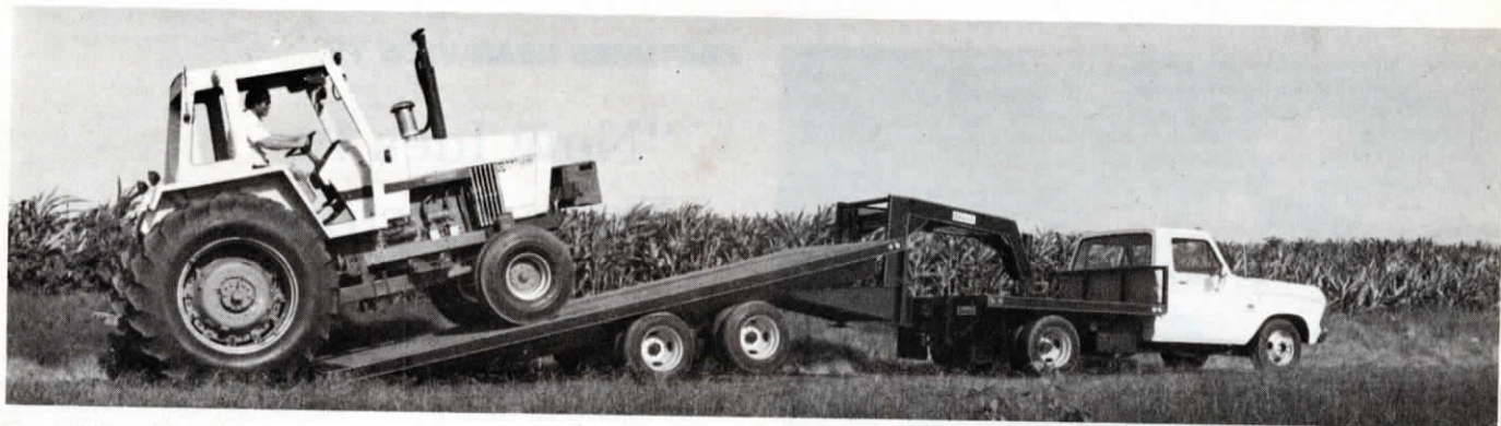
Dump/Tilt trailer tilts on a "gentle incline" for easy drive-on loading, and unloading, of machinery and equipment.
