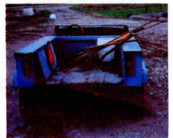
Box has removeable endgate. Tail lights were salvaged off an old pickup.
