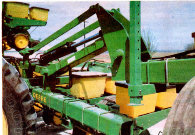
Hinges are first welded in place on toolbar and then toolbar is cut.
