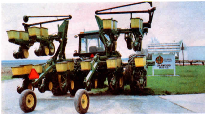
Weld-on kit can be installed on any 7 by 7 or 5 by 7 rigid toolbar without even removing the row units. Row units remain parallel to the ground when folding.
