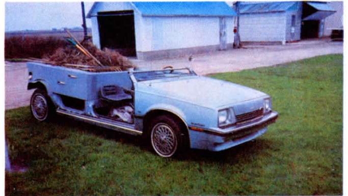
Kalkwarf turned a 1982 Chevrolet Cavalier front wheel drive station wagon into a chore pickup that'll haul up to 800 lbs. of cargo at a time.
