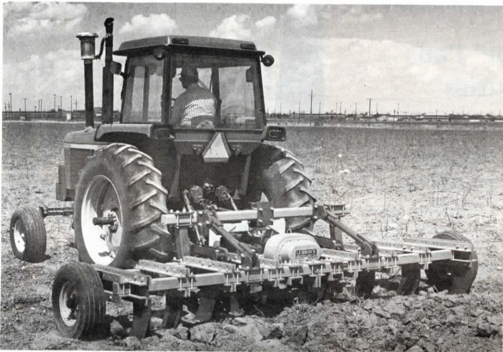
New oscillating 3 pt. hitch acts as an insulator which prevents vibrations from being transferred to the tractor.
