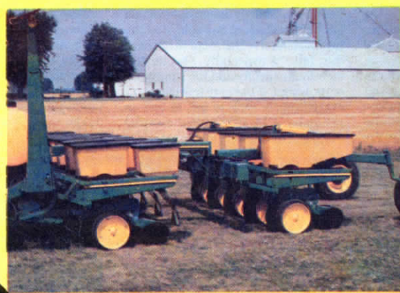
The new add-on "Splitter" rides independent of the forward planter. Many different row combinations are possible.
