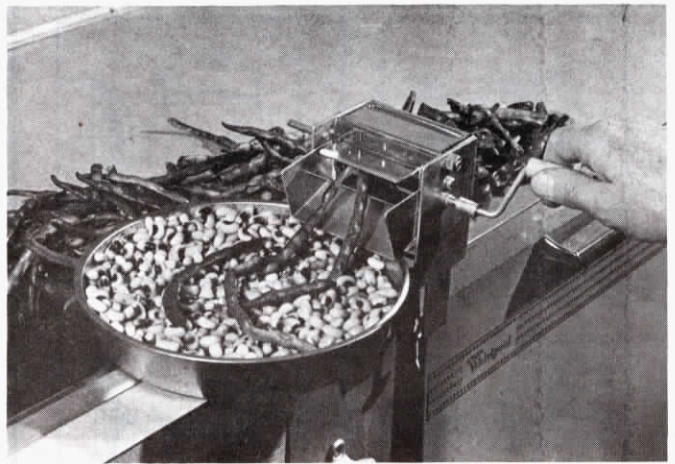
You can hook a portable electric mixer up to the drive shaft of the hand-crank pea sheller.
