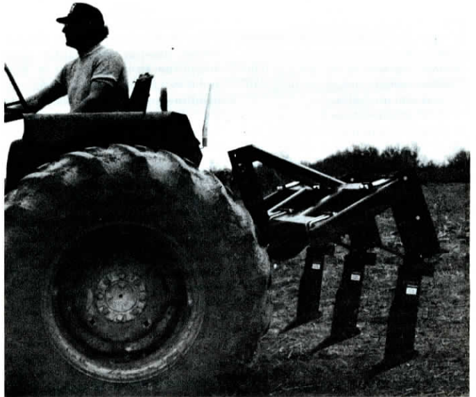
Sub-Mulcher toolbar models are available in 3, 4, 5 and 7 shank models, all with 3 pt. hitch hookup.
