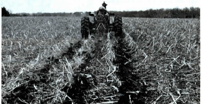
A popular method of using the Sub-Mulcher is to run it over corn stalks in the fall after harvest. When it penetrates the soil, it cuts, lifts and fractures the soil up to 20 in. on either side without mixing subsoil and topsoil.
